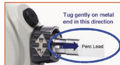
I After the pump restarts, rotate the perc lock on the new controller in the direction of the "locked" icon until the perc lock clicks into the fully-locked position. If unable to engage perc lock to the locked position, gently push the driveline into the controller to assure a proper connection. Retry to engage perc lock.
